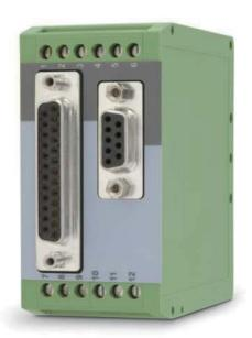
Suitable for operation with sensors and encoders using SSI interface Converts SSI data as well as serial data to parallel data format Parallel output 25 bits (push-pull, short-circuit proof)
