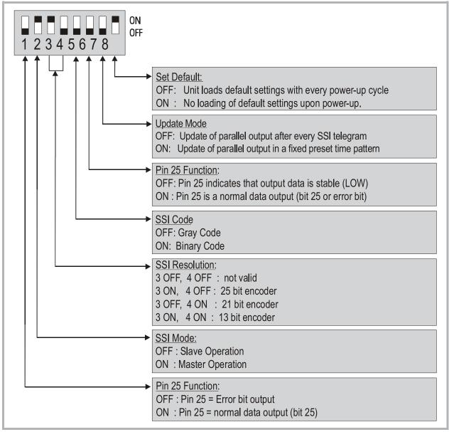
The switch settings shown in the example are suitable for Master operation of a 25 bit SSI encoder with Gray coded output. The parallel output operates with equidistant update times and pin 25 is used to indicate valid and stable output data.
