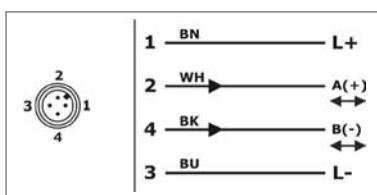
4-wire, RS485 Modbus RTU Conductor color standard connection cable M12 – A-coded: BN = brown, WH = white, BU = blue, BK = black
