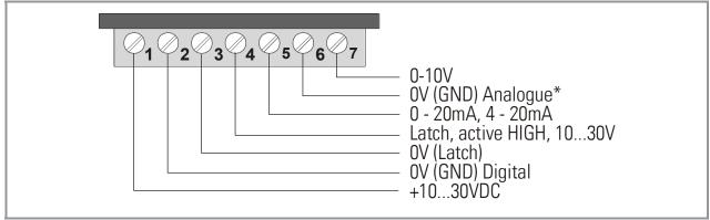
\* Potential separated from GND digital/ power supply (terminal 2)
